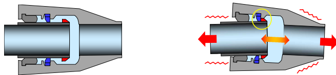
Fig.8 Earthquake-resistant joints... Structure that does not cause joint detachment during the earthquake (Left: Normal Condition, Right: Earthquake Condition)
