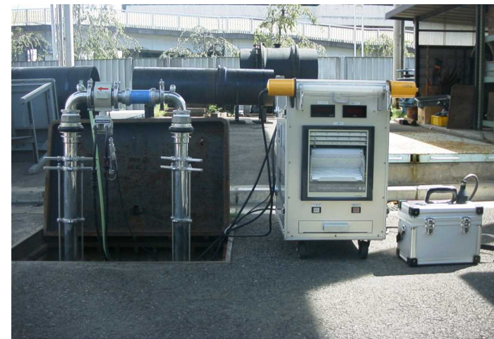
Fig.20 Minimum flow meter
