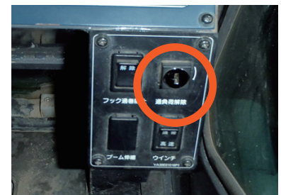
Keyhole for releasing the overload protector
