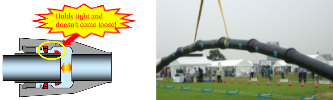
Figure 1 Structure of seismic resistant coupling-fitted pipes, and demo of hanging connected pipes
