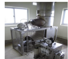
Figure 4. The Tokyo Waterworks Artificial Rainfall Device
