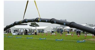
Figure 1: Responds to movements in the ground such that the joints do not come loose.
