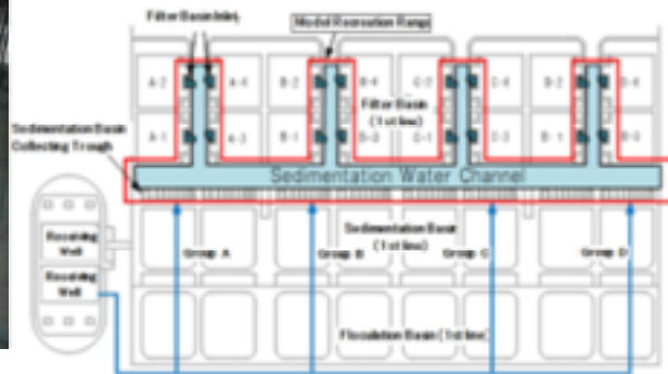
Figure 8 Hydraulic model experiment recreation range
