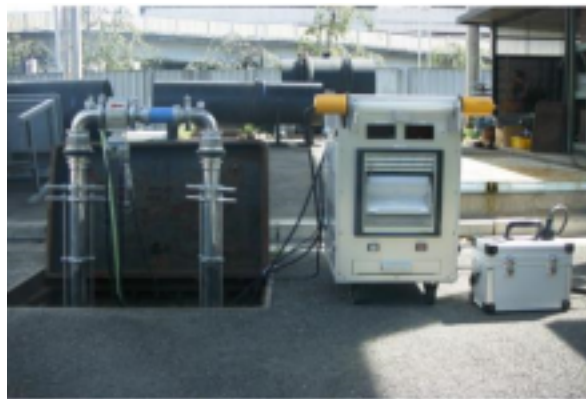
Figure 4 Minimum Flow Rate Measurement Device
