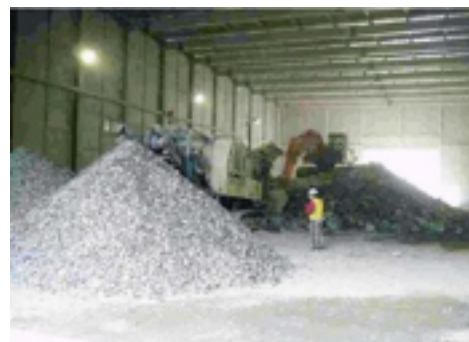
Fig. 7: Production of the recycled aggregate made using removed bomb-protection layer materials
