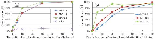
Figure 4 (a) Removal of MCs and AT-a by sodium hypochlorite (Add MCs and AT-a to ultrapure water (Experiment No. 2); (b) Add MCs to raw water in Ozaku purification plant (Experiment No. 3))
