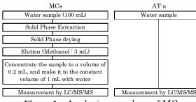
Figure 1 Analysis procedure of MCs and of AT-a
