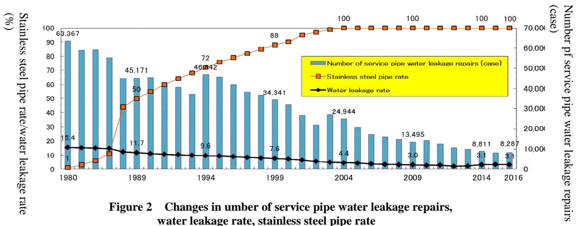
Figure 2 Changes in number of service pipe water leakage repairs, water leakage rate, stainless steel pipe rate
