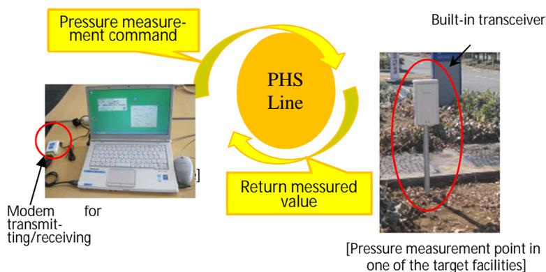
**Figure 5** Collection of water pressure data
