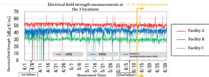
**Figure 11** Communication test and electrical field strength
