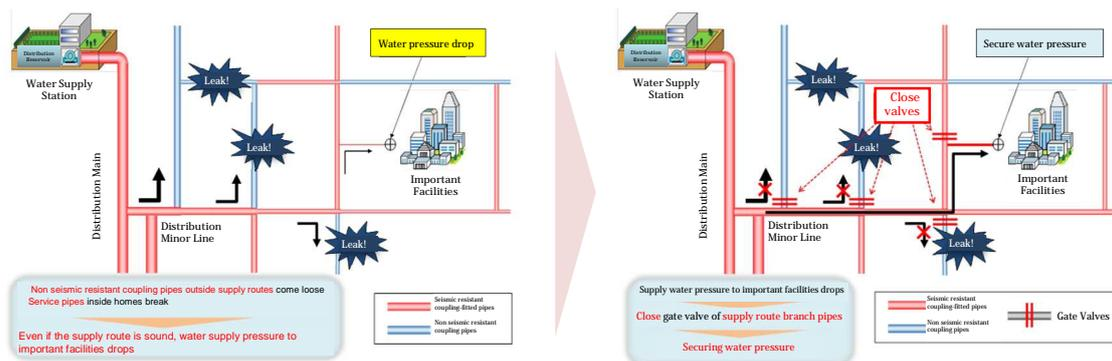
**Figure 3** Conceptual image of securing water pressure to important facilities
