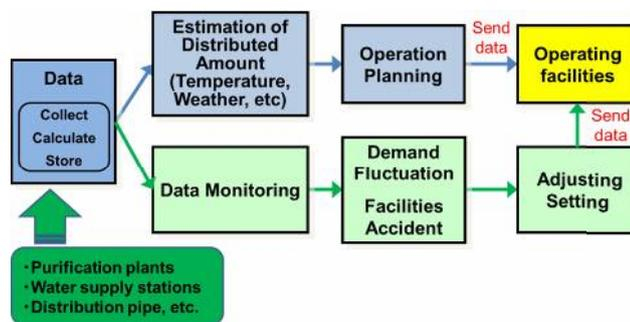
Figure 4 Roles of the Water Supply Operation Center
