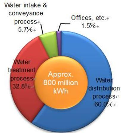
Figure 2 Breakdown of electricity usage
