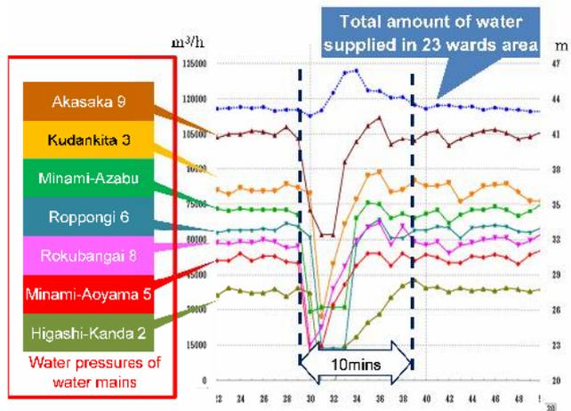
**Figure 11** Changes of water supply and water pressure during the Kumamoto earthquake
