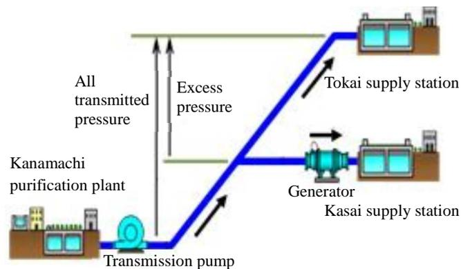
**Figure 2** Status of excess pressure at Kasai
