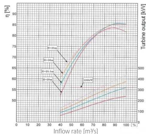
**Figure 5** Characteristic curve of power generation efficiency
