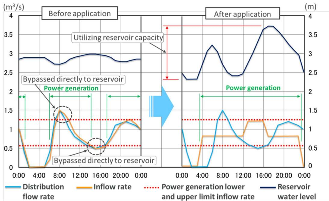
**Figure 3** Changes in distribution reservoir operation
