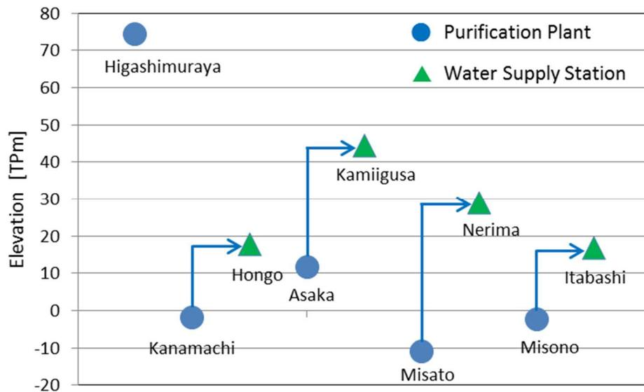
Figure 3: Differences in elevation between water purification plants and water supply stations
