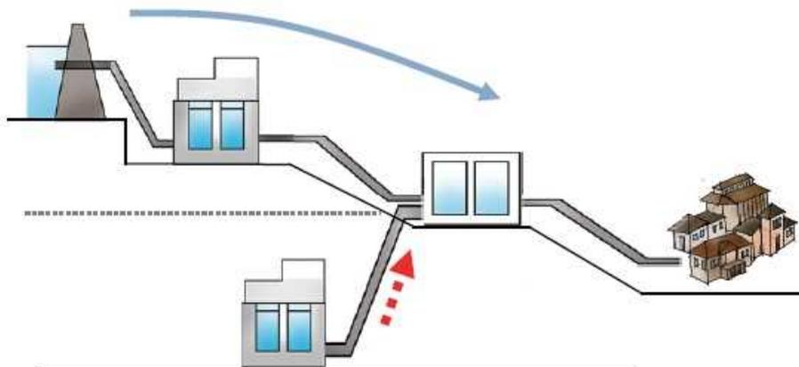
Figure 7: Water transmission utilizing gravity flows
