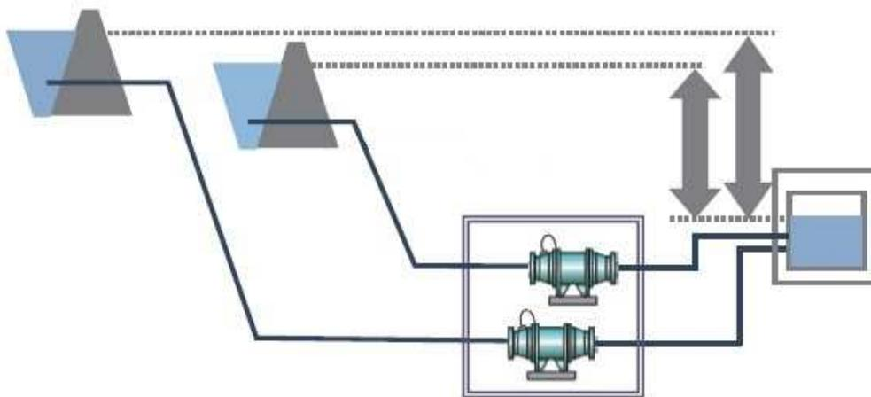
Figure 6: Small-scale hydroelectric power generation utilizing altitude differences
