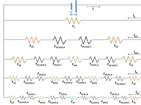
Figure 2 Electric Equivalent Circuit
