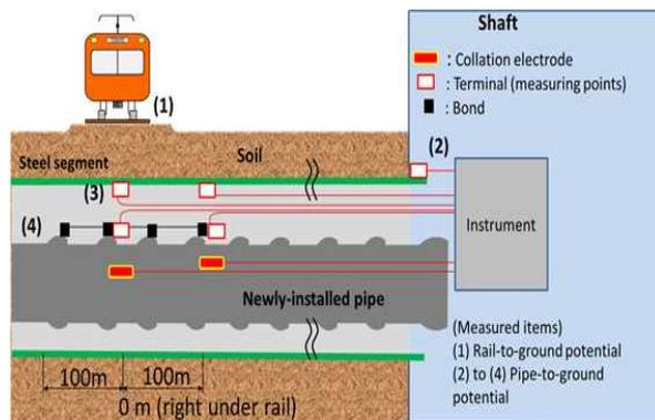
**Figure 5** Measurement system from the actual field survey
