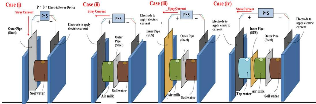
**Figure 4** Experiment Circuit diagram simulating each case
