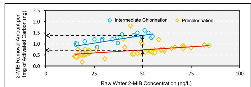
Figure 5. Difference of Removal Effect of 2-MIB by Chlorination Method
