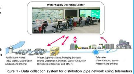
Figure 1 - Data collection system for distribution pipe network using telemeters
