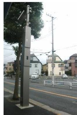
Figure 8 - Telemeter with combined casing/lead-in pole
