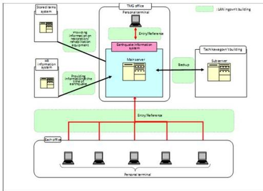
Earthquake information system configuration diagram
