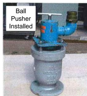
Picture 6. With a ball pusher installed
