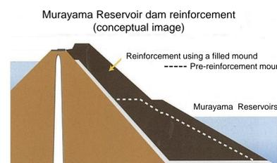
Figure 11: "Tangible" measures -Reservoir dam reinforcement work-
