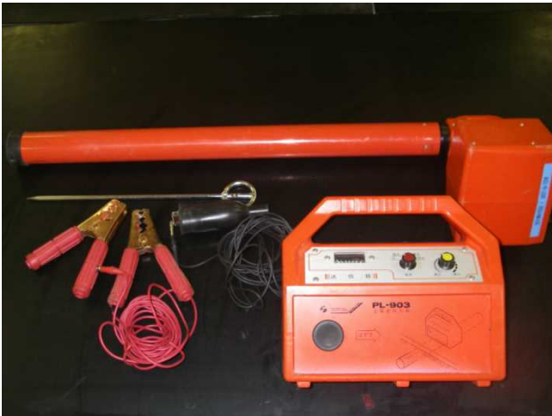
Fig.23 Metal pipe detector
