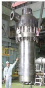
Boiler circulation pump for thermal power plant [India]
