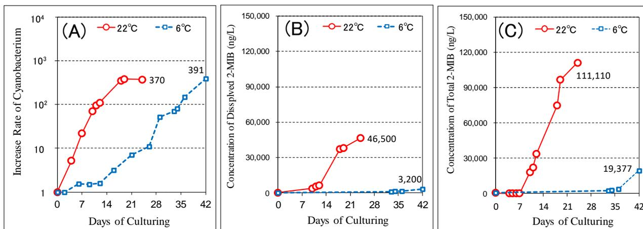
**Figure 6.** Change in Increase Rate of *P. autumnale*, Concentration of 2-MIB in a Dissolved Form and Concentration of Total 2-MIB at High and Low Water Temperatures
