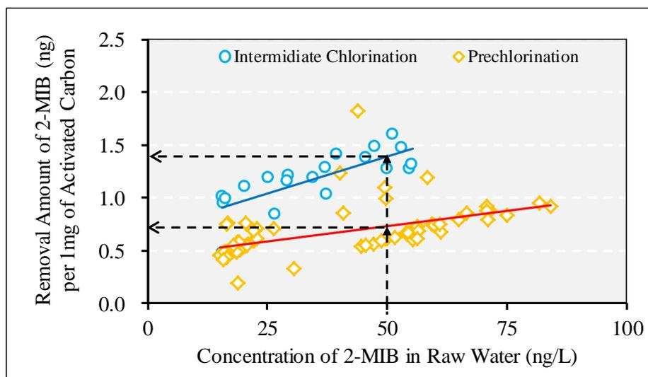
**Figure 7.** Quantities of 2-MIB removal per 1 mg of powdered activated carbon (A comparison of pre- and post-implementation of intermediary chlorination)
