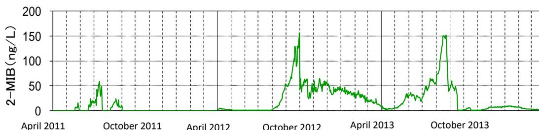
**Figure 2.** Transition of 2-MIB Concentration in Raw Water at Ozaku Purification Plant (at 9:00 am)
