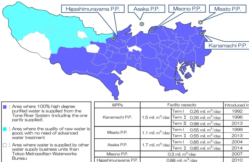
**Figure 2** WPPs with advanced water treatment installed and their capacity
