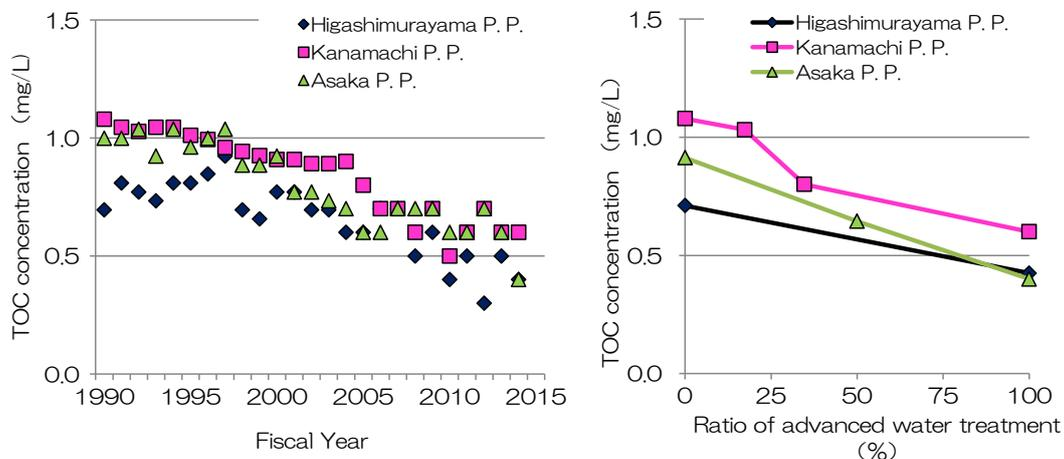
**Figure 5** Change of TOC concentration after the implementation of advanced water treatment
