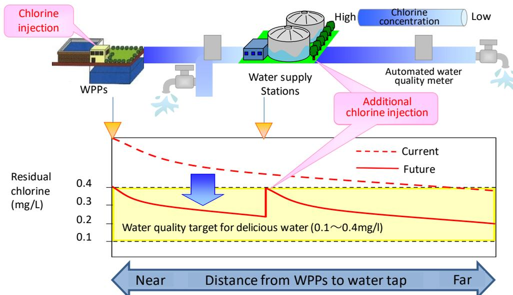
**Figure 3** The effect of additional chlorine injection facilities
