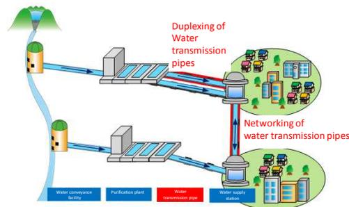
Figure 4 Duplexing and networking of water transmission pipes
