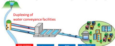
Figure 3 Duplexing of water conveyance pipes
