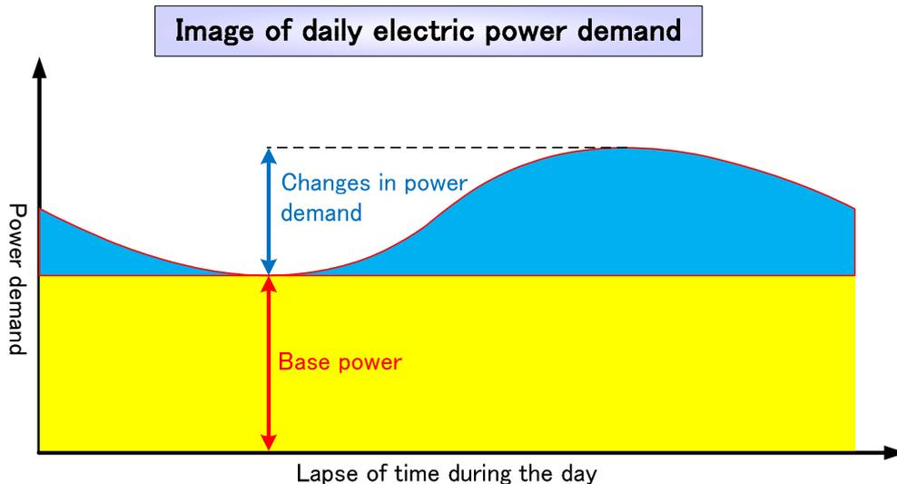
However, their intended purpose is entirely different. While emergency generators have been installed assuming the operation while commercial power supply is discontinued, continuous generators in plants of BWTMG are basically intended to work continuously to supply base power<sup>V</sup> and rely on commercial power for fluctuation of power demand.
