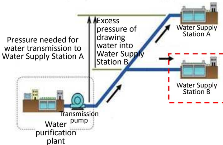
**Figure 1: Excessive drawing pressure at Water Supply Station**
