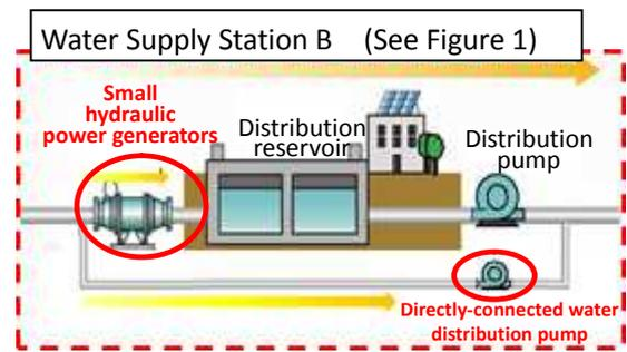
**Figure 2: Energy saving equipment utilizing excessive drawing pressure at Water Supply Station**
