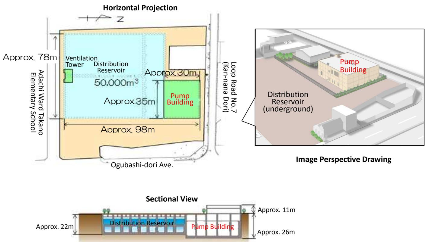
**Figure 5: Layout of Kohoku Water Supply Station**
