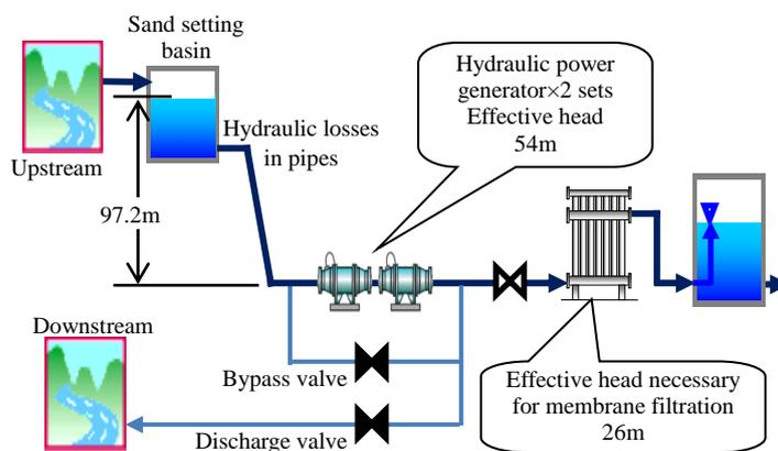
**Figure 10** Serial connection of hydraulic generators and discharge
