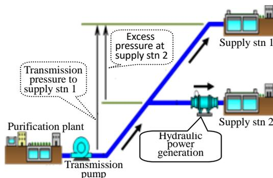
Figure 12 Using excess pressure
