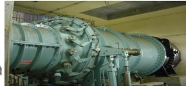
**Figure 8** Hydraulic turbine
