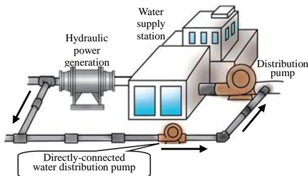
Figure 14 Hybrid energy saving system
