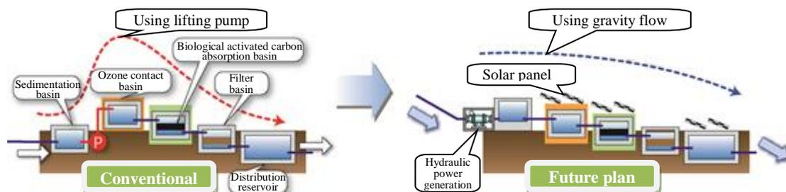
**Figure 17** Utilization model of renewable energy
